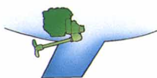
MS2B-V (V-reverse gear) Propeller shaft, 20 degree angle Reverse engine installation
